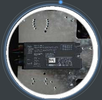
Driver DALI-2 / D4i, NFC hors tension
