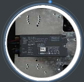
Driver DALI-2 / D4i, NFC hors tension
