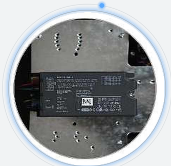
Driver DALI-2 / D4i, NFC hors tension
